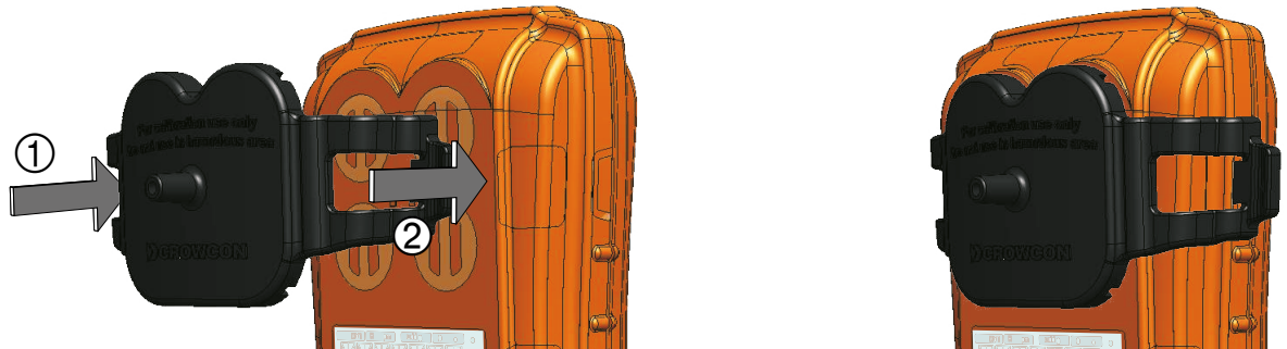
Figure 5: Fitting the calibration/bump test plate
